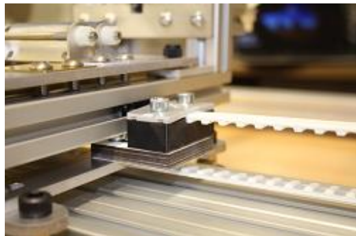
Figure 31: Toothed belt tension
