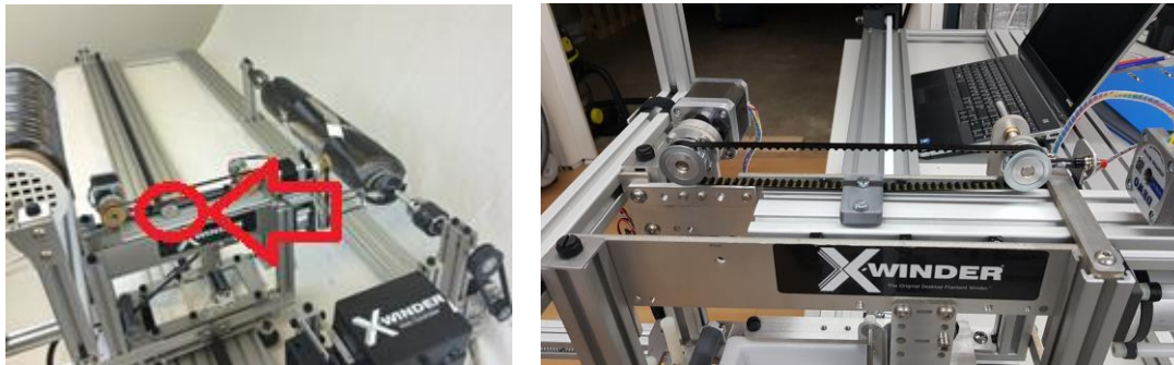
Figure 35: Mounting the rotation head
