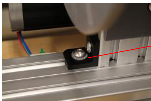
Figure 28: assemblage du mandrin
